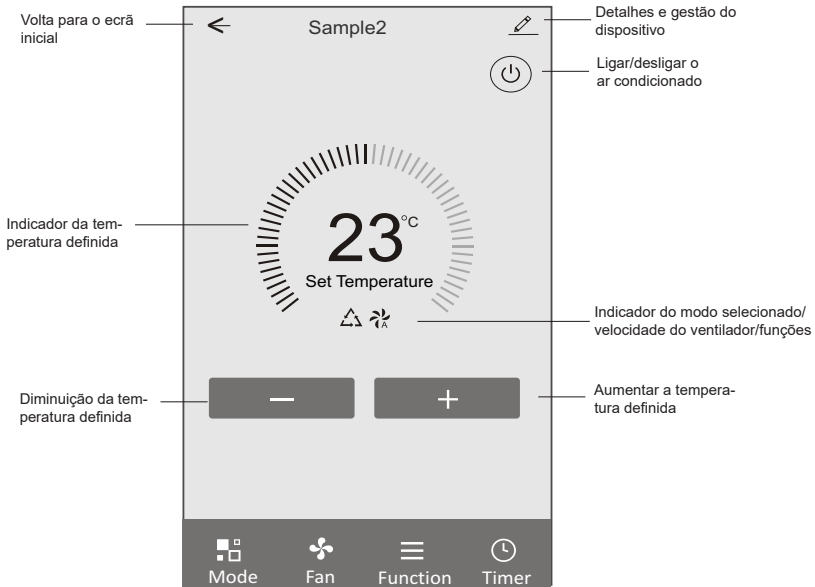
A interface de controlo principal
