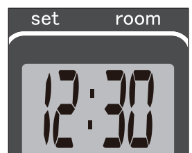
F: When the 4-digit stops blinking, the setting has been locked to the indicated value.
