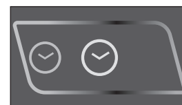
H: The TIMER indicator light indicates that the timer function has been switched on.
