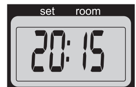
F: When the 4-digit stops blinking, the setting has been locked to the indicated value.
